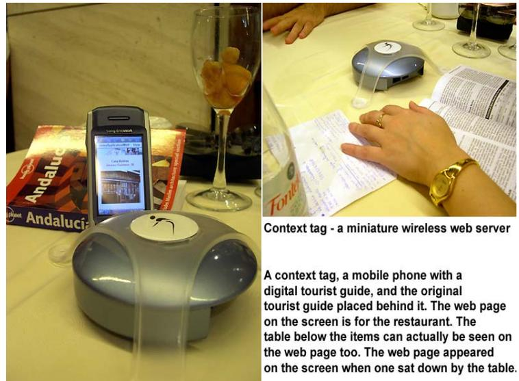
Figure 0. Tag and mobile device
